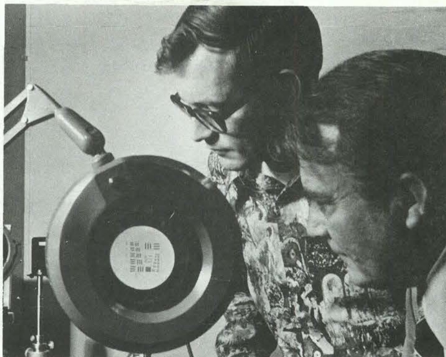
IMAGE RESOLUTION of new PFE device is checked by inventors Paul Peery (5112) and Cecil Land (5133). The new method of storing images in PLZT ceramics eliminates the need for layers of photoconductive film on ceramic.
